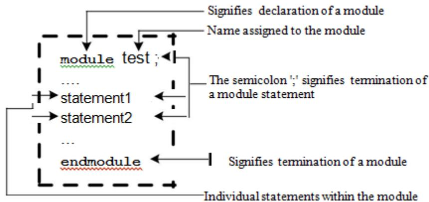
Figure 2 Structure of a typical simulation module.
