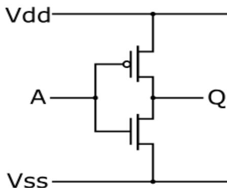
Figure 1 CMOS inverter
